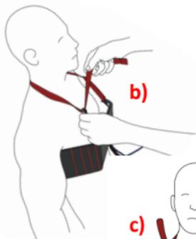
**b)** Attach the carabiner hooks to the slots in the NCCD plate [2] as shown in image b) and c).
