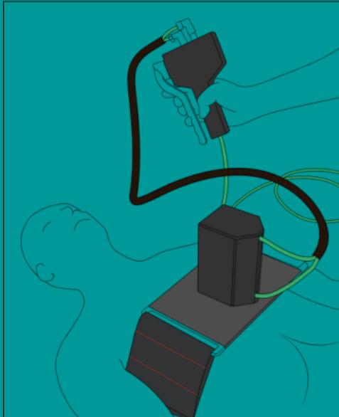
NCCD is a compact, lightweight chest compression device to be used as a substitute to manual chest compression during CPR. NCCD is powered by compressed gas, and designed for use in hyperbaric environments.
